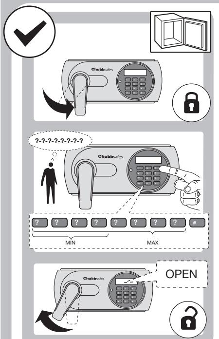
**GB** To check that your PIN code has been accepted operate the lock three times without closing the door. If unsure repeat the steps above.
